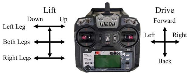
Fig. 8 Joystick control strategy: The right stick controls the drive DOF, moving the robot in four different directions (forward, backward, left, and right). The left joystick controls the lift DOF, moving the target leg up or down. The vertical axis of the left stick is used to select which side's coxa is adjusted.
